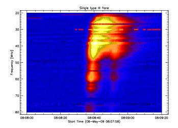
**Fig. 4.** Two low-frequency isolated type III solar radio bursts observed at Bleien observatory, Switzerland. Antenna = logarithmic-periodic CLP-5130.
