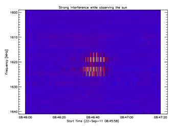
Fig. 41. Fast moving IRIDIUM satellite in the L-band near 1620 MHz observed at Bleien observatory Switzerland.
