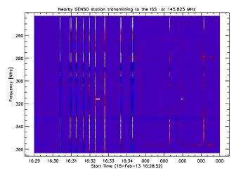
Fig. 31. Sporadic harmonics/cross-talk from strong amateur radio communication (GENSO) in 2m band.
