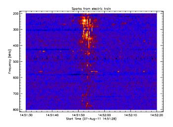
**Fig. 25.** Quasi burst caused by a nearby electric train (SOB). Antenna = log-per, linearly polarized.
