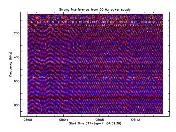
Fig. 51. Wobbling cords (50 Hz)due to a cheap, overloaded power supply.
