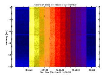
Fig. 47. Calibration steps generated by an adjustable attenuator from 0 dB in steps of 1 dB up to 10 dB) applied to low frequency Callisto. Intensity bars yellow=hot, red=warm and blue=cold.
