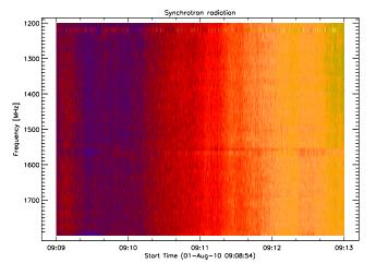
Fig. 12. Gyro-synchrotron solar radio radiation observed in Lband at Bleien observatory, Switzerland. Antenna = 5m dish, linearly polarized, pointing to sun.
