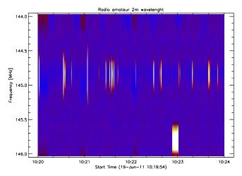
**Fig. 30.** Sporadic NFM (narrow frequency modulation) from amateur radio communication (HAM) in 2m band.
