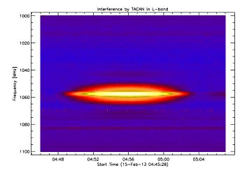
Fig. 44. TACAN signal form aircraft at 1057 MHz observed with Callisto on a 5m dish at Bleien observatory Switzerland.
