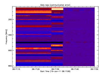
Fig. 48. Twice data loss near 08:17:30UT due to inappropriate resources of an old PC.
