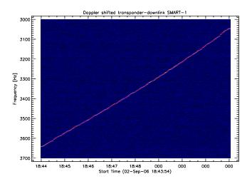
**Fig. 24.** Weak transponder signal from SMART-1 in its perilunar orbit. Antenna = 5m dish, linearly polarized.
