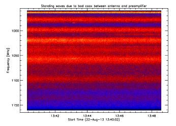
Fig. 53. Interference introduced by unmatched components in the high frequency path (SWR).
