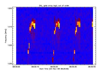
Fig. 21. Interference due to damaged gate array logic in the front-end of the telescope observed at Bleien observatory, Switzerland. Antenna = parabolic dish 5m, linearly polarized  $45^{\circ}$ .
