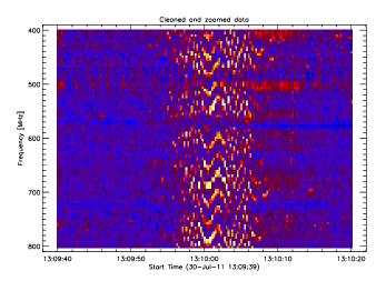
**Fig. 26.** Necklace burst man made by a lawn cutter. Antenna = log-per, linearly polarized.
