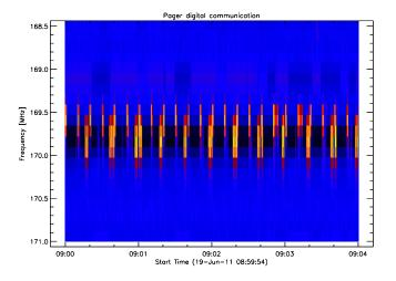
Fig. 33. Permanent communication in NFM-FSK (narrow band frequency frequency shift keying.
