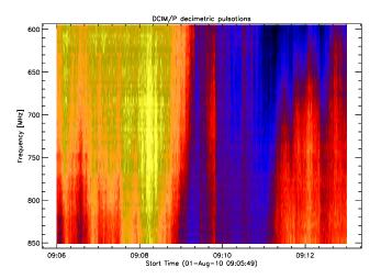
**Fig. 10.** DCIM (decimetric) solar radio burst with continuum observed at Bleien observatory, Switzerland. Antenna = 7m dish, circularly polarized LHCP, pointing to sun.
