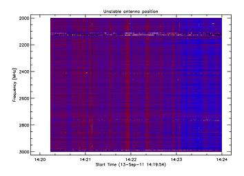
**Fig. 50.** Flux fluctuations (vertical stripes) in the S-band observed at Bleien observatory Switzerland with FFT-spectrometer Phoenix-3.
