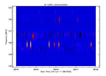
Fig. 29. Sporadic AM (amplitude modulation) from air traffic communication.
