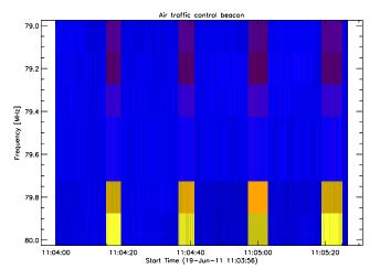
Fig. 27. Beacon of local airport used for radio-navigation. Period about 20 seconds with high transmission power.
