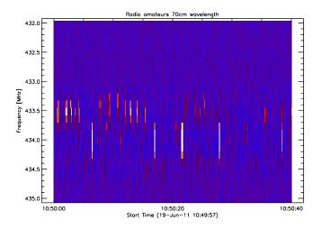
Fig. 37. Sporadic NFM (narrow frequency modulation) from amateur radio communication (HAM) in 70cm band.
