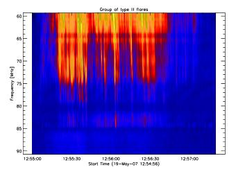
**Fig. 5.** Group of type III solar radio bursts observed at Bleien observatory, Switzerland. Antenna = log-per CLP-5130, linearly polarized. Some type III are reverse drifting.
