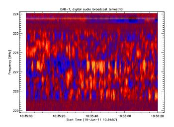
**Fig. 34.** Permanent (24h/7d) communication in DAB-T (digital audio broadcast terrestrial).
