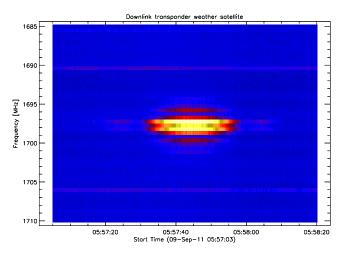
**Fig. 42.** Fast moving weather satellite in the L-band near 1697 MHz observed at Bleien observatory Switzerland .
