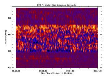
Fig. 38. DVB-T (digital video broadcast terrestrial, a permanent transmission in broad band technology.
