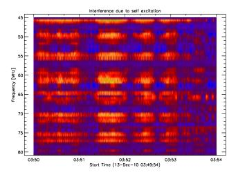
Fig. 49. Self excited system due to bad shielding and high gain amplifer.
