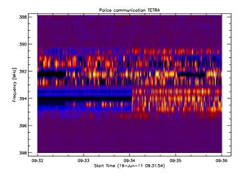
Fig. 36. TETRA, permanent communication 24h/7d in digital broad-band transmission.
