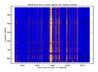
Fig. 52. Strong rfi produced by badly filtered sewing machine.
